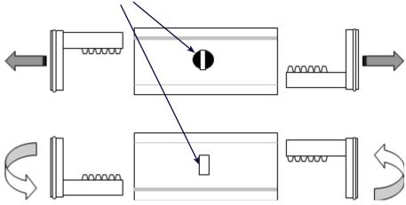
**Rotate pistons and re-insert.** Note: Before engaging the piston (gear rack) with the pinion, "Back Rotate" the pinion gear by one tooth for proper orientation.
