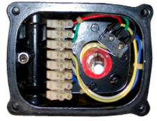
The **NEXUS-LS**<sup>™</sup> Limit Switch with Standard Indicator Cap for 90° flow paths.
