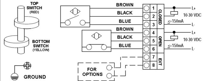
P3A = Proximity Sensors NPN NC (3-Wire) Inductive Sensors
