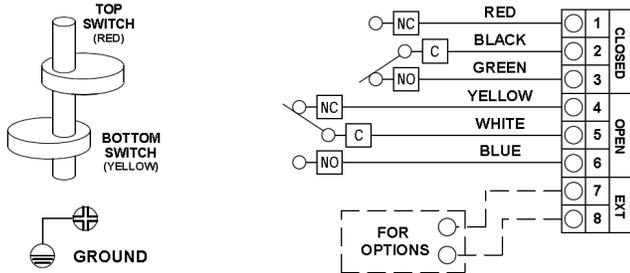
M2A = Mechanical Switches 2 SPDT (Standard)
