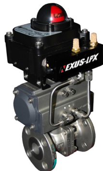
NEXUS-LPX™ Discrete Valve Controller shown with aero2 actuator & SVF B41C ANSI Class 150# Flanged Ball Valve. (Shown with optional stainless steel tubing)
