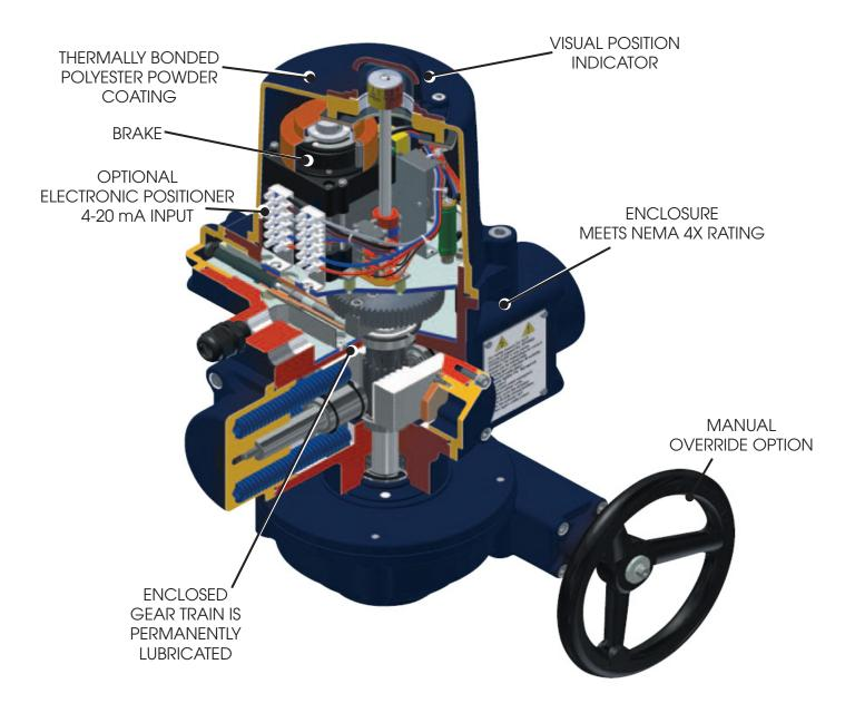
Sample Specification based on "SR" Series Model ESR50V4MXCM (ESR Series, 443 in-lbs, NEMA 4X, 115 VAC 50% Duty Cycle, Fail Closed, 4-20mA Control Package with Manual Override).
