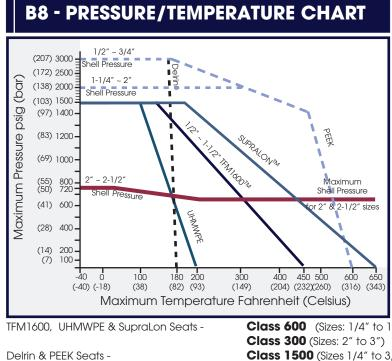
\* For sizes 1/4" and 3/8" refer to "Series R8 Ball Valve" Data Sheet \*\* At full differential pressure for clean fluids with TFM1600™ Seats
